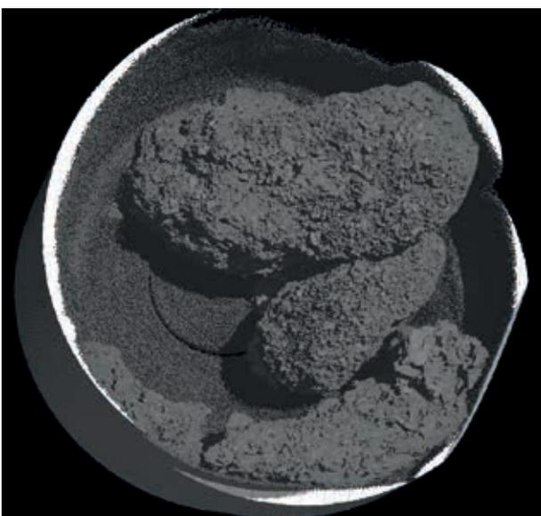
**Fig. 9:** Rendering of the box after stressing the low signal in the histogram. Ring artifacts are visible in the CT image due to the low signal-to-noise ratio.
